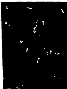
F Photoelectrons produced by X rays of wavelength 1.5 Å
